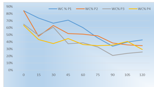
Figure 2. Water content variation with time in the four piles during the composting process
