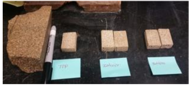
Figure 4. Eolianite cross-sections cut into dominos .
