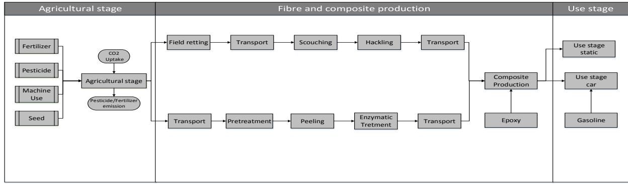
**Figure 1.** System boundaries of the LCA study. All the foreground process for the different scenarios are included.
