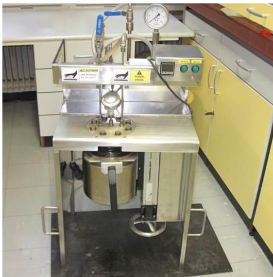
Figure 1: Laboratory scale high pressure, high temperature reactor.
