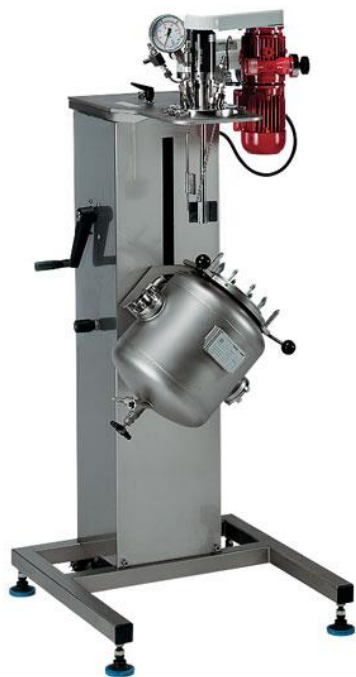
Figure 2: Pilot high pressure and high temperature plant.
