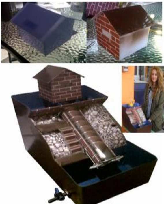
Figure 10. The Educational Renewable Energy Screw Wheel for Pico Hydropower Generation.
