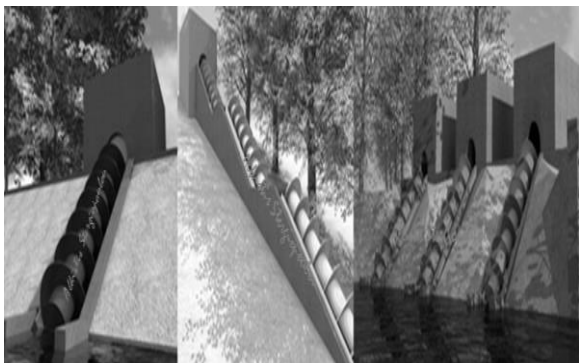
Figure 2. Photorealistic artistic views for one Archimedean Screw, three screw in series and three screws in parallel, made by A. Stergiopoulou
