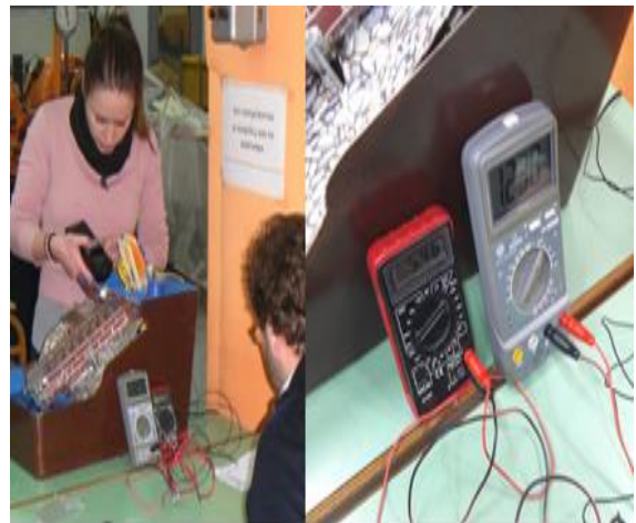
Figure 11. Current and voltage measurements with two multimeters and rotation speed measurements with an electronic handle rotation meter
