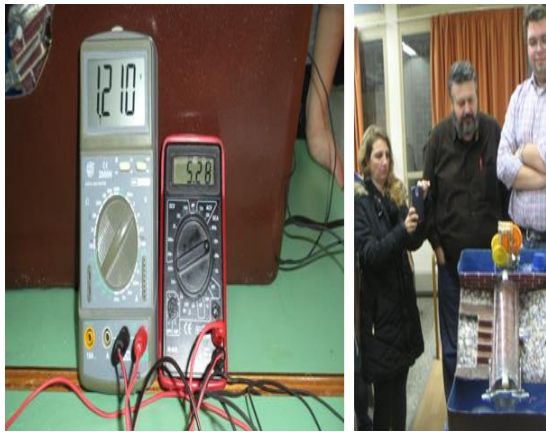
Figure 12. Measuring voltage and current (f.e. V=1.210 V and I=5.28 mA)
