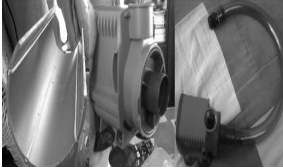
Figure 8. Plastic shroud of the rotor and two views of the pump
