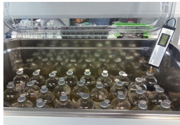
Figure 1 BMP assay experimental set up
