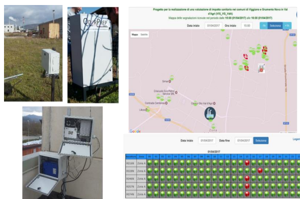
Figure 3: PID, electronic nose, OdorPrep and an example of OdorLab network
