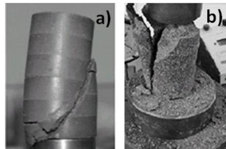
**Figure 2.** UCS samples a) lime-treated; b) PSA-treated
