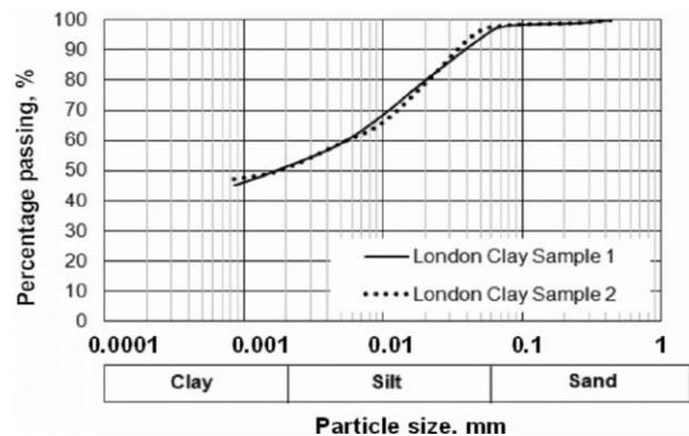
**Figure 1.** Particle size distribution of London clay
