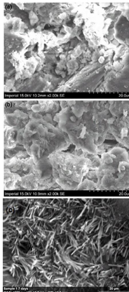
**Figure 3.** Indicative SEM results: (a) untreated soil; (b) 4% lime-treated soil; (c) 14% PSA-treated soil
