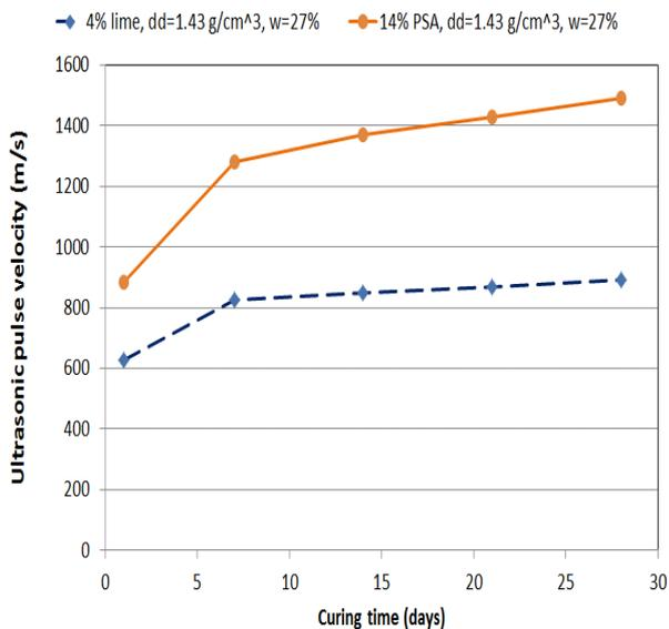
**Figure 7.** Indicative PUNDIT results (air-cured samples)
