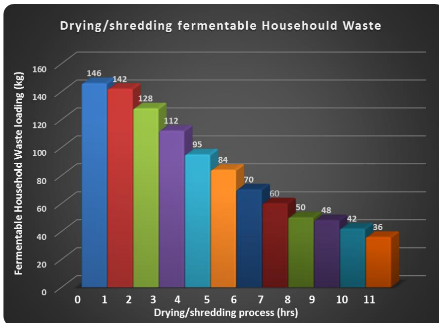
Figure 3. Evolution of the weight for a typical Fermentable Household Waste loading (kg) vs Drying/shredding processing time (hrs).
