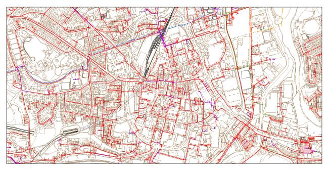
**Figure 1.** Map of in-use (red bold lines) and abandoned (purple bold lines) low pressure gas pipelines in the city centre of Huddersfield, retrieved from the GIS database of Northern Gas, the gas network manager (Map scale 1:5000)
