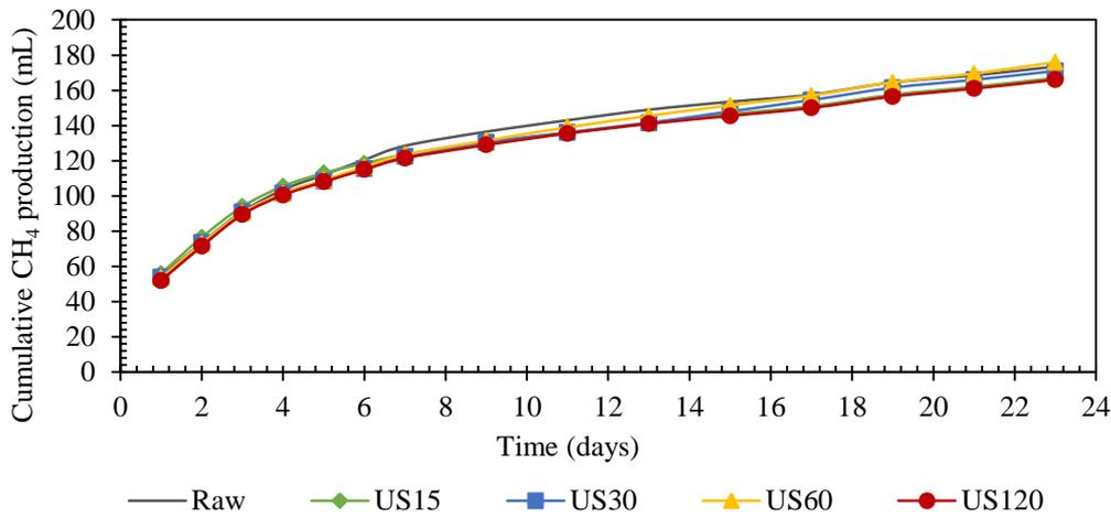
**Figure 3.** Cumulative methane production
