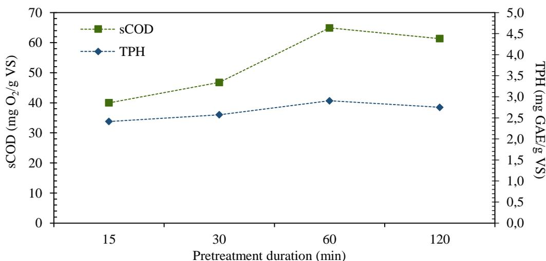
**Figure 2.** Effect of ultrasound pretreatment on sCOD and TPH concentrations
