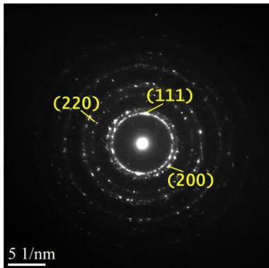
**Figure 2.** SAED pattern of thin Au-Fe film
