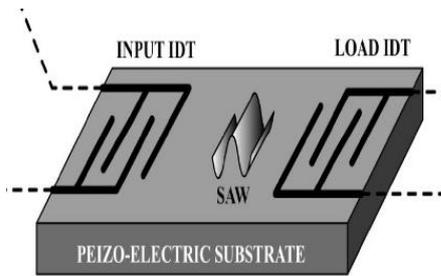
**Figure 6.** The concept of integrated nano-piezo-device for energy harvesting
