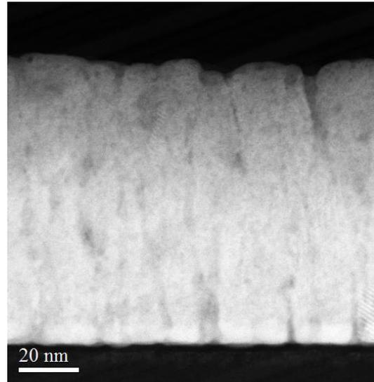
**Figure 4.** STEM image of thin Au-Fe film
