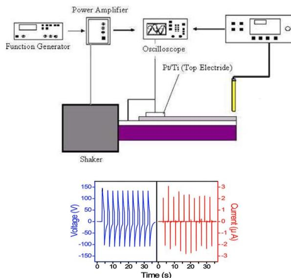
**Figure 10.** Test stand for piezo-electric evaluation
