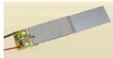
**Figure 9.** Prototype of integrated nano-piezo-device
