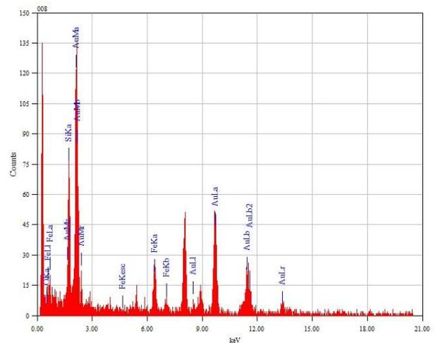
**Figure 5.** EDS spectra of thin Au-Fe film
