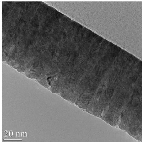
**Figure 1.** CTEM image of thin Au-Fe film
