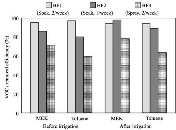
**Figure 3.** Results summary of gaseous VOCs removal
