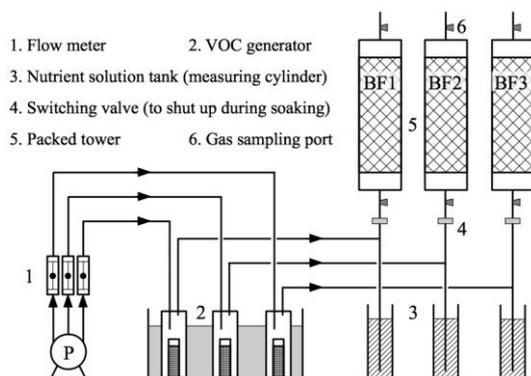
**Figure 1.** Experimental setup of biofiltration
