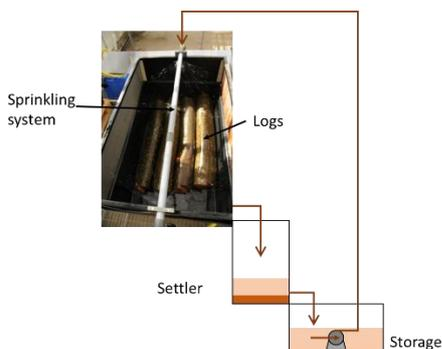
**Figure 1.** Pilot scale sprinkling system
