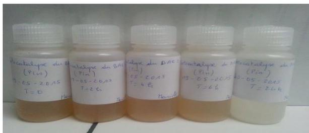
**Figure 8.** Decolorization during photocatalysis for spruce
