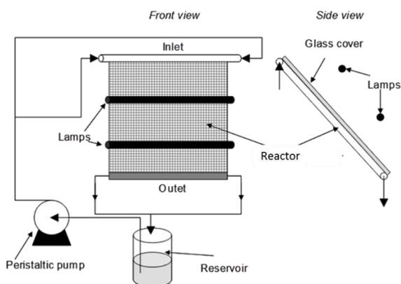
**Figure 2.** Photocatalytic reactor
