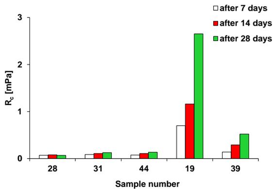
Figure 1. Resistance to one-axial compression ( $R_c$ ) of dense mixtures based on fly ash from coal combustion in pulverized coal boilers (28 – C-PFA; 31,44 – NC-PFA) and in fluidized-bed boilers (19, 39 – C-FFA)
