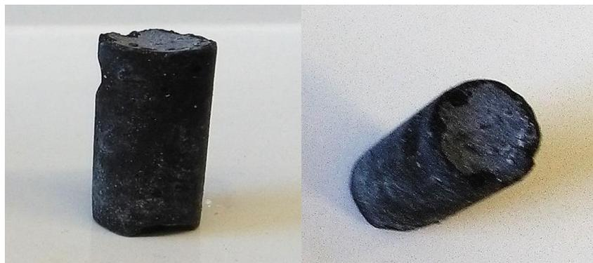
**Figure 1.** Geopolymer obtained from biomass ash
