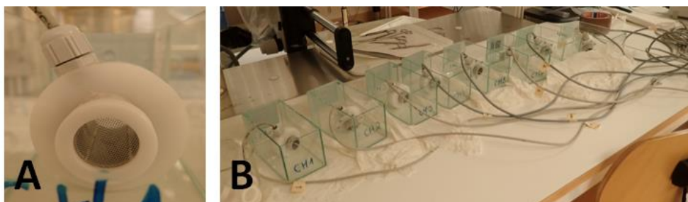
Figure 1. MFB test chamber for a single animal exposure (A), and the set of the experimental aquaria used for simultaneous measurements with 8 channels (B). The measurement principle is based on the animal functioning as resistant in an alternating current between electrodes at opposite walls of the test chamber. Movements of the animal change the conductivity and the electrical field between a second, non-current carrying pair of electrodes and generate specific electrical signals for different kinds of behavior (swimming, locomotion, etc.).
