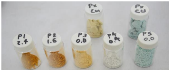
Figure 6. Precipitates. From the leachate after accelerated weathering laboratory runs (lower row); precipitates from an operating mine (upper row)
