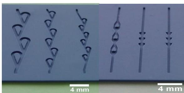
**Figure 6.**Microfluidic elements within LTCC layers
