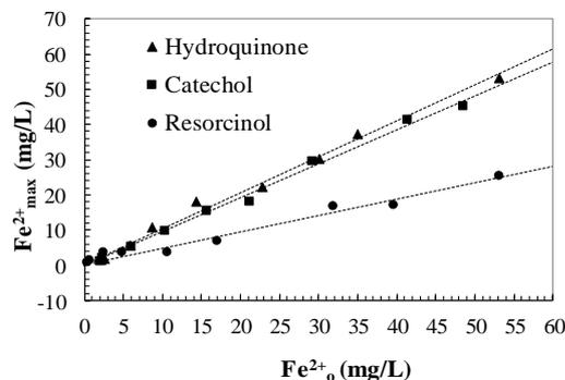
**Figure 4.** Concentration of dissolved ferrous ions when oxidized samples show maximum turbidity. Experimental conditions:  $C_o=100.0$  mg/L;  $\text{pH}=3.0$ ;  $\text{H}_2\text{O}_2=4.0$  mM;  $T=25.0^\circ\text{C}$ .
