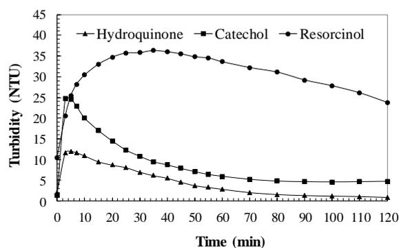
**Figure 1.** Changes of turbidity during the oxidation of phenolic compounds by Fenton reagent. Experimental conditions:  $C_0=100.0$  mg/L;  $\text{pH}=3.0$ ;  $\text{H}_2\text{O}_2=4.0$  mM;  $\text{Fe}=20.0$  mg/L;  $T=25.0^\circ\text{C}$
