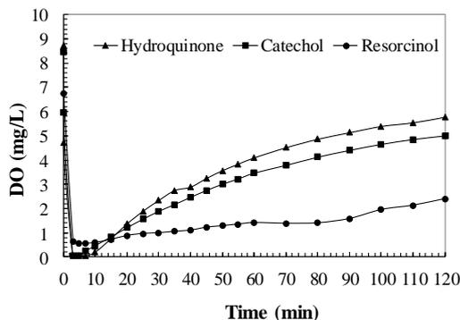
**Figure 2.** Changes of dissolved oxygen (OD) during the oxidation of phenolic compounds by Fenton reagent. Experimental conditions:  $C_0=100.0$  mg/L;  $\text{pH}=3.0$ ;  $\text{H}_2\text{O}_2=4.0$  mM;  $\text{Fe}=20.0$  mg/L;  $T=25.0^\circ\text{C}$ .
