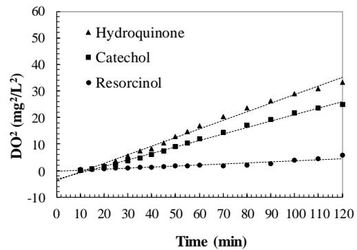
**Figure 3.** Second order kinetics of dissolved oxygen formation during the oxidation of phenolic compounds. Experimental conditions:  $C_0=100.0$  mg/L;  $\text{pH}=3.0$ ;  $\text{H}_2\text{O}_2=4.0$  mM;  $\text{Fe}=20.0$  mg/L;  $T=25.0^\circ\text{C}$ .
