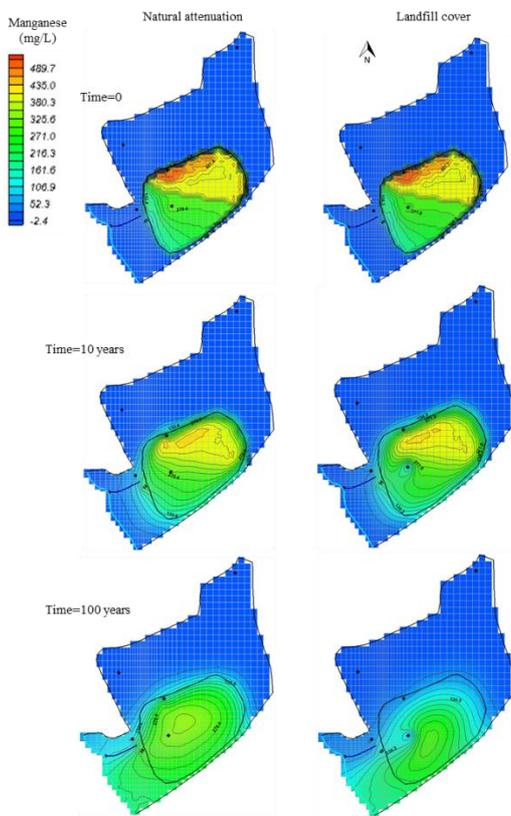
**Figure 4.** Simulation results for manganese concentrations in groundwater in a summer situation.
