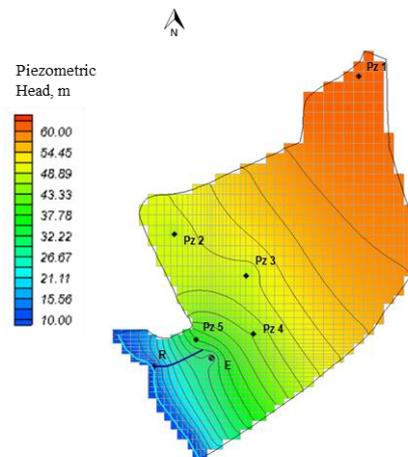
**Figure 3.** Simulation results for piezometric heads in a summer situation.
