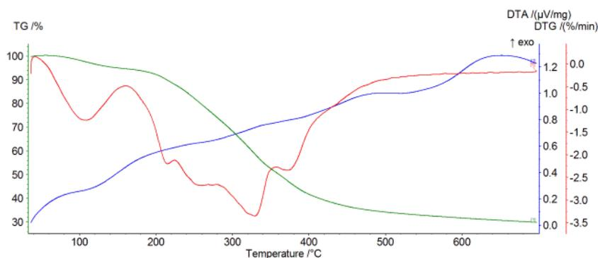
**Figure 4.** Thermal analysis of biomass samples: A) straw waste, B) rape residue
