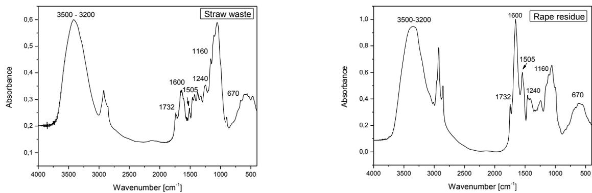
**Figure 2.** Infrared spectra of straw waste and rape residue
