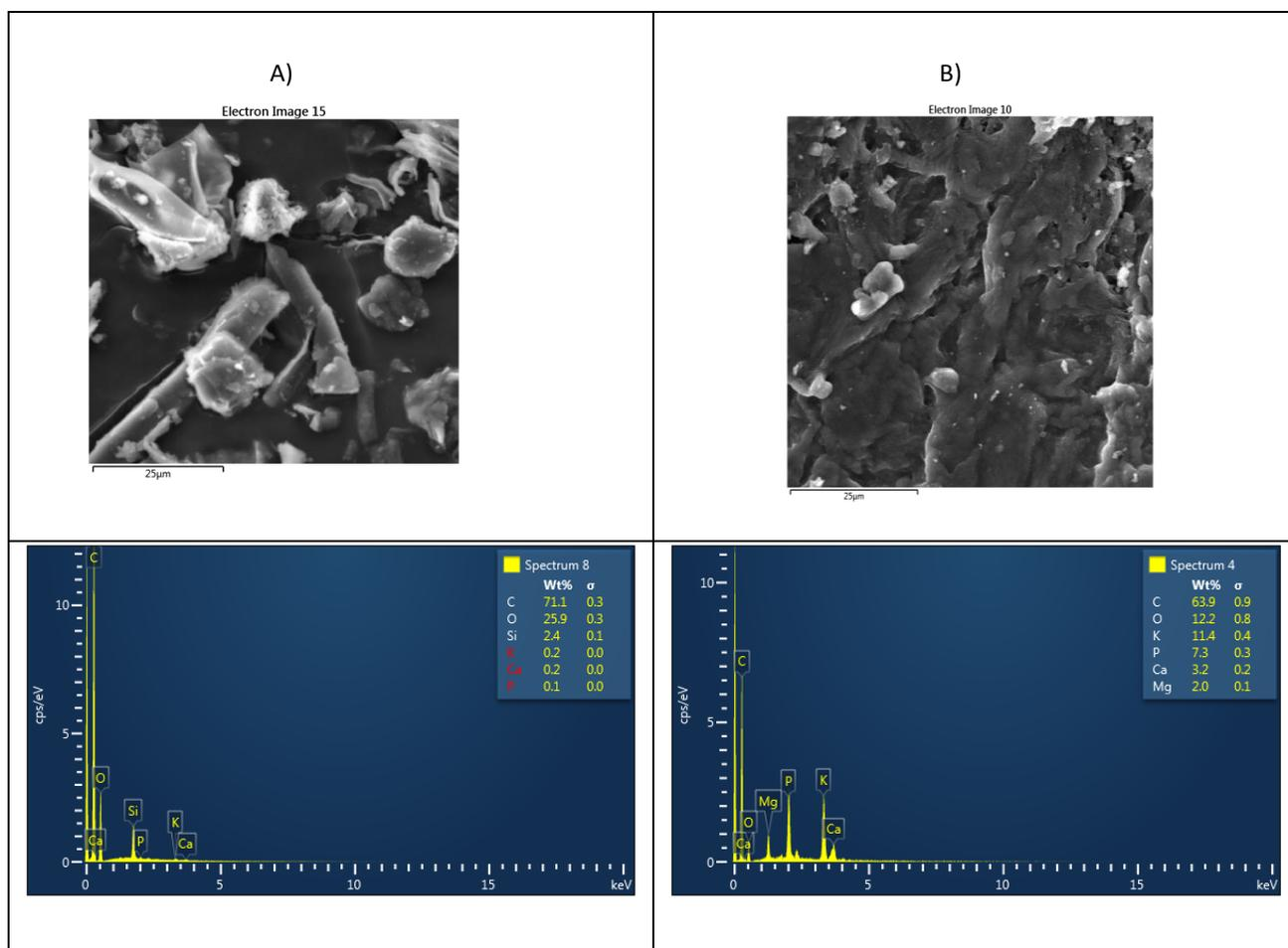
**Figure 3.** SEM-EDS spectra of biomass samples: A) straw waste, B) rape residue
