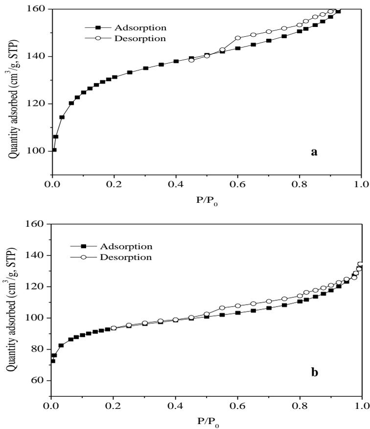
**Fig. 1** N<sub>2</sub> adsorption and desorption isotherms of AC (a) and BC (b)
