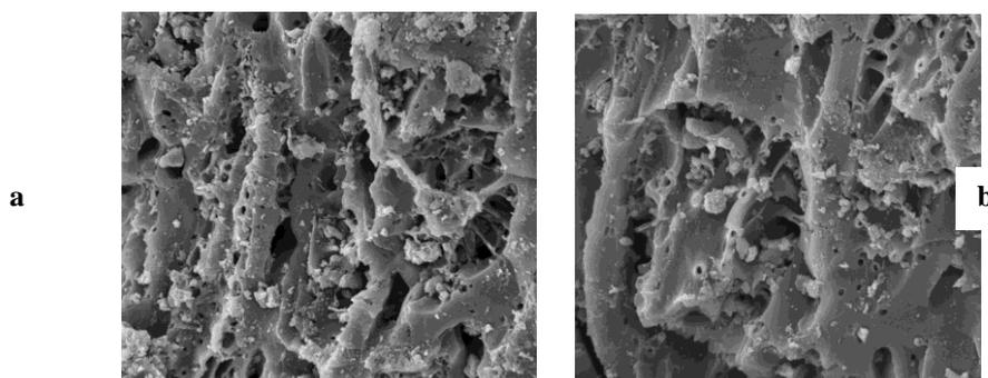
**Fig.3** The scanning electron microscopy images of BC before (a) and after (b) adsorption
