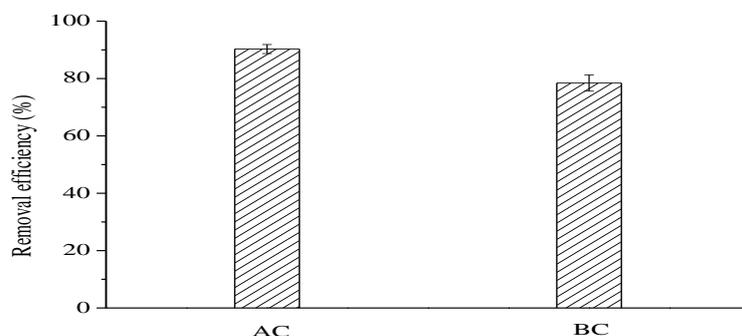
**Fig. 2** H<sub>2</sub>S adsorption performances of AC and BC adsorbents
