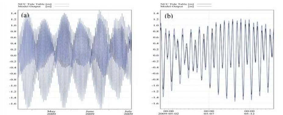
**Figure 6.** Comparison of the observed and simulated water surface elevation at Ab Shirin Kon station, (a) for 3 months, from mid-April to mid-July 2009 (model runtime), (b) for fifteen days, from early-May to mid-May 2009
