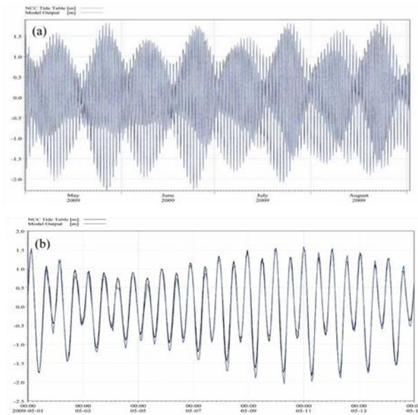
**Figure 5.** Comparison of the observed and simulated water surface elevation at Bandar Abbas station, (a) for 3 months, from mid-April to mid-July 2009 (model runtime), (b) for fifteen days, from early-May to mid-May 2009
