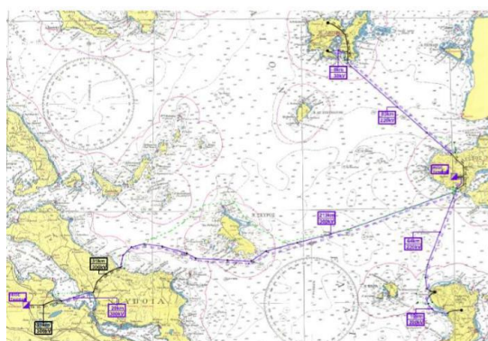
Figure 10: Submarine power transmission plans (source: ROKAS Renewables)
