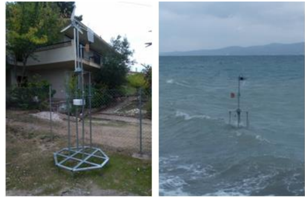
Figure 15: Wind and Wave Application Experimental (pilot) Device developed by the SEALAB [16]
