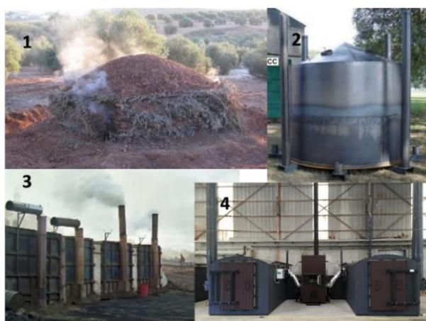
Figure 1: Charcoal production technologies as investigated in this paper: (1) mould earth kiln; (2) metal ring kiln; (3) Missouri type kiln; (4) modern metal kiln with gas recycling
