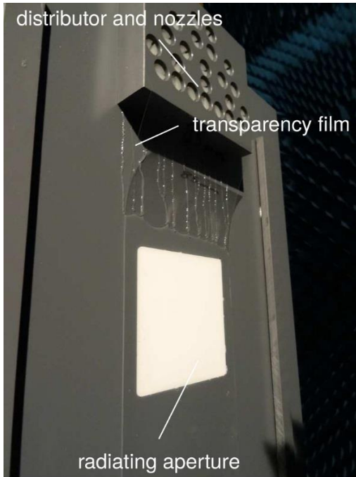
Figure 3. Close-up of the horn antenna mounted in the sprinkler. The white square in the middle is the radome (polystyrene) of the antenna and the grey area is made of polyvinyl chloride (PVC). The sprinkler nozzles distribute the water flow and the membrane (polyester) generates a thin water film coating the radiating aperture.
