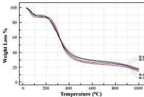
**Figure 1.** TGA curves of EPS from different media (K1: dissolved EPS in LB, K2: particulate EPS in LB medium, K5: dissolved EPS in LB+whey, K6: particulate EPS in LB+whey).
