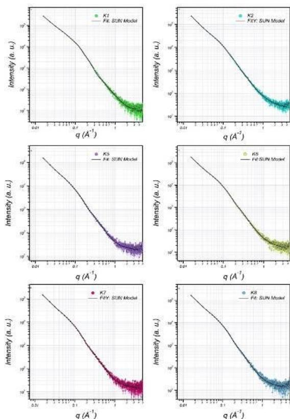
**Figure 3.** The SAXS data are fitted (solid curves) using lamellar + prolate core shell model (K1: dissolved EPS in LB medium; K2: particulate EPS in LB, K5: dissolved EPS in LB+whey, K6: particulate EPS in LB+whey, K7: dissolved EPS in LB+Glukoz, K8: particulate EPS in LB+Glukoz)
