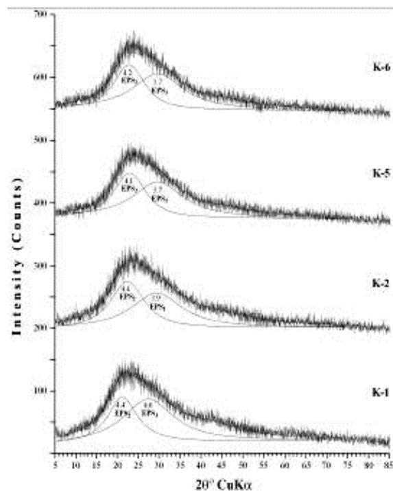
**Figure 2.** XRD patterns of EPS from different media. (K1: dissolved EPS in LB medium, K2: particulate EPS in LB medium, K5: dissolved EPS in LB+whey, K6: particulate EPS in LB+whey).
