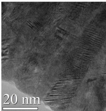
**Figure 3.** CTEM image of thin Au-Fe film at high magnification
