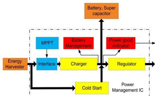
**Figure 12.** Concept for harvester energy management
