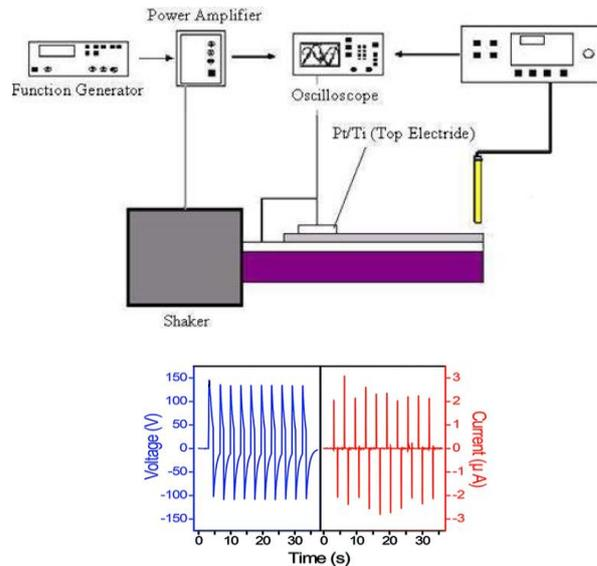
**Figure 10.** Test stand for piezo-electric evaluation
