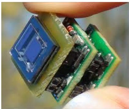
**Figure 11.** Piezoelectric device, PZT type
