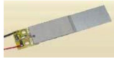
**Figure 9.** Prototype of integrated nano-piezo-device
