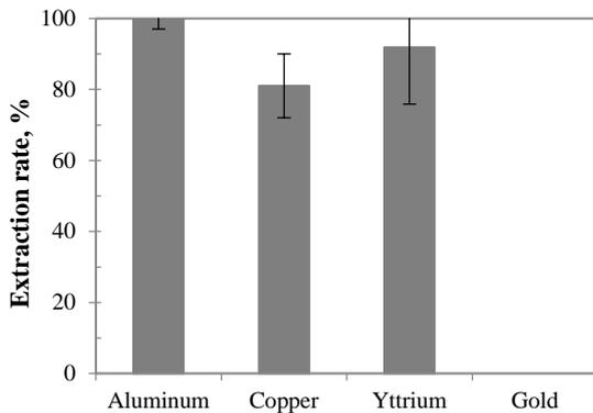
**Figure 2.** Extraction rates for the selected metals during sulfuric acid leaching
