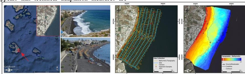
**Figure 1.** Kamari beach (Santorini): (a) location, the beach and the backing coastal wall/road; (b) survey grid lines, sediment samples, and location of the camera and hydrodynamic observation (ADV) stations, and (c) beach topography/nearshore bathymetry.
