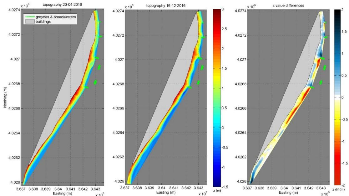
**Figure 3.** Beach topography in 20-4-2016 (left) and 16-12-2016 (middle). Beach sediment changes (on the basis of the beach topographic surveys) is shown at the right panel.
