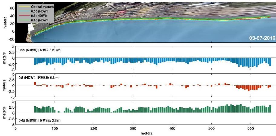
**Figure 5.** Comparison between shoreline detections from satellite imagery using 3 different values of the normalized difference water index-NDWI (0.45, 0.5, 0.55) with the shoreline detections from the coastal video imagery for the georectified mosaic of 3/7/2016. The smallest RMSE (0.8 m) is found when the MDWI is set at 0.5.
