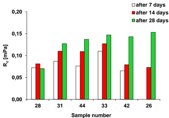
Figure 2. Effect of fuel on the resistance to one-axial compression ( $R_c$ ) of dense mixtures based on fly ash from coal combustion in pulverized coal boilers (28 – C-PFA; 31,44 – NC-PFA; 33, 42 – BC-PFA; 26 – GC-PFA)
