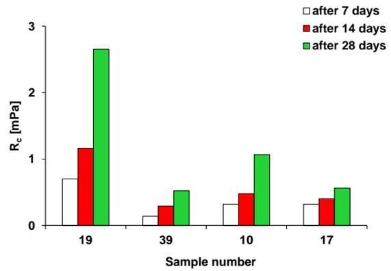
Figure 3. Effect of fuel on the resistance to one-axial compression ( $R_c$ ) of dense mixtures based on fly ash from coal combustion in fluidized-bed boilers (19, 39 – C-FFA; 10, 17 – B-FFA)
