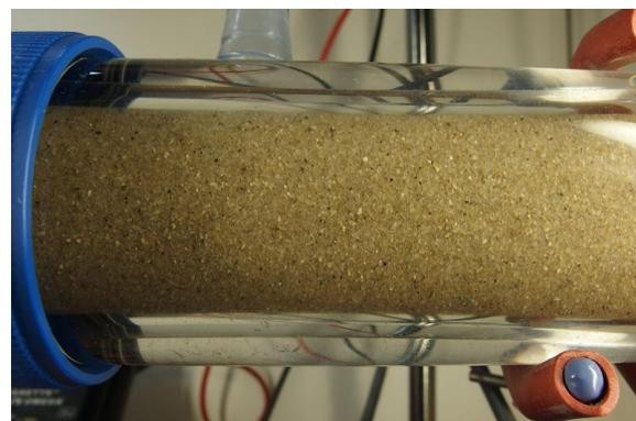
**Figure 3.** Photograph of the 1<sup>st</sup> part of the column (entry) at the start (1<sup>st</sup> cycle) of surfactant flushing.
