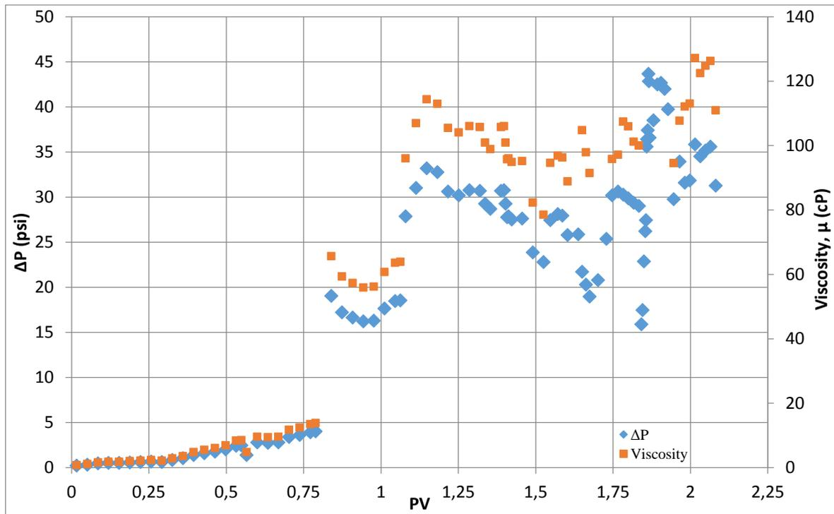
**Figure 2.** The differential pressure between inlet/outlet of the column is shown for the surfactant flood: 0,25PV surfactant injected followed by 0,25PV of air. The pressure drop was used to compute the apparent viscosity, which was calculated about 60 cP after the 3rd cycle and increased to 100cP during the 7th cycle
