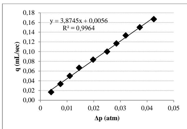
**Figure 1.** Pressure drop  $\Delta p$  [atm] measured for a range of flow rates and then used to compute the hydraulic conductivity and permeability of the pack.
