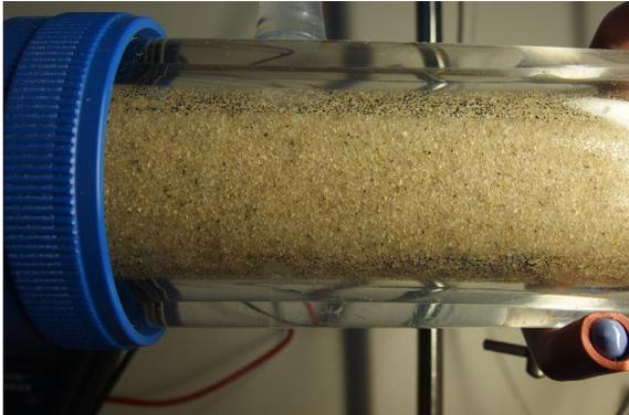
**Figure 4. Photograph** the 1<sup>st</sup> part of the column (entry) at the end of the 7<sup>th</sup> cycle of surfactant and air flushing – foam visible (after 3 days).
