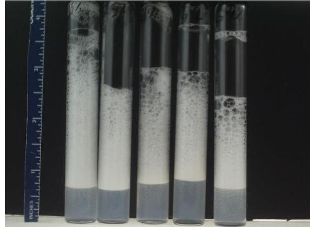
**Figure 2.** Preliminary foam “shake” test comparing five formulations to select the best foamer.
