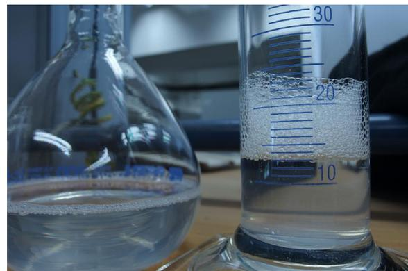
**Figure 5.** Foam collected from the exit of the column after being shut-in for 3 days as a proof of foam stability.
