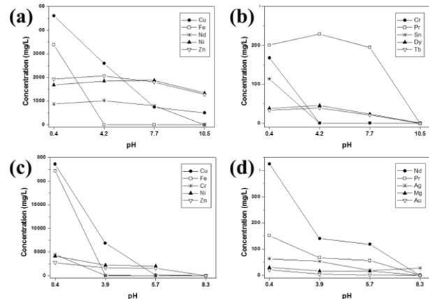
**Figure 4.** ICP-AES analysis of the supernatant at different pHs : (a) camera-major elements, (b) camera-minor, (c) PCB-major elements, (d) PCB-minor elements
