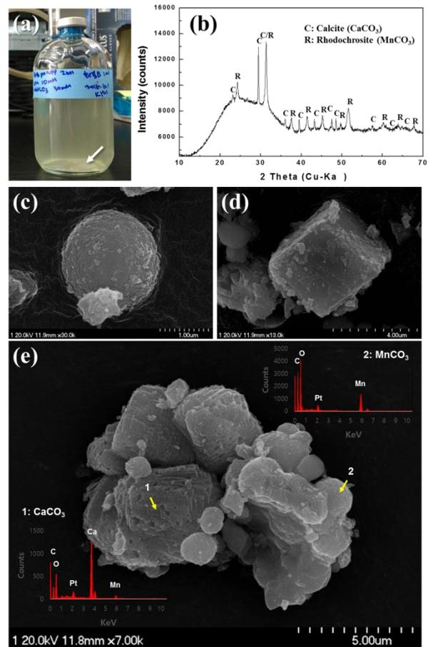
**Figure 6.** A picture showing the white settled precipitate (a), XRD patterns (b), SEM-EDS images of biogenic carbonate minerals (c-e).
