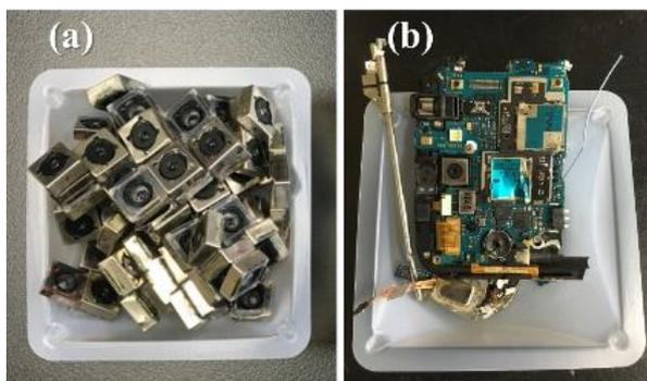
**Figure 1.** Camera and PCB parts separated from mobile phone waste
