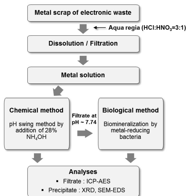
**Figure 2.** The process to separate and recover metals including Fe, Cu, and rare earth-metal complex from mobile phone waste by combining chemical and biological methods.
