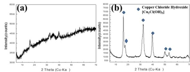
**Figure 3.** XRD patterns of the precipitate separated from the camera metal solution at pH 4.2 (a) and pH 7.7 (b).
