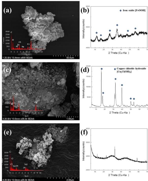
**Figure 5.** SEM-EDS images and XRD patterns of precipitate separated from the PCB metal solution at pH 3.9 (a,b), pH 5.7 (c,d) and pH 8.3 (e,f).
