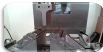
Figure 2. Application of the three point bending test
