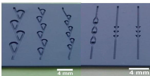
**Figure 6.**Microfluidic elements within LTCC layers
