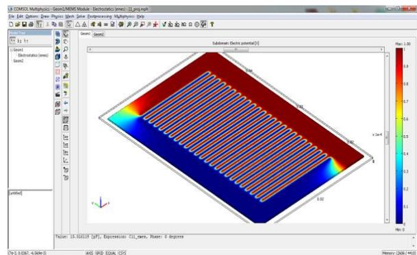
**Figure 4.**Simulation of interdigit sensor and capacitance response
