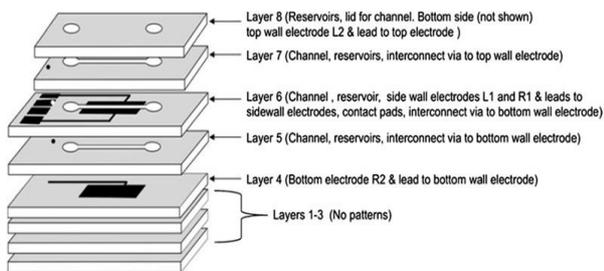
**Figure 5.**Embedding microfluidic features as tailored LTCC layers
