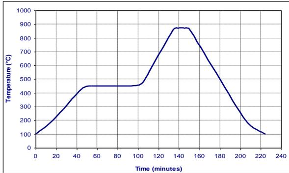
**Figure 2.**Example of LTCC firing process
