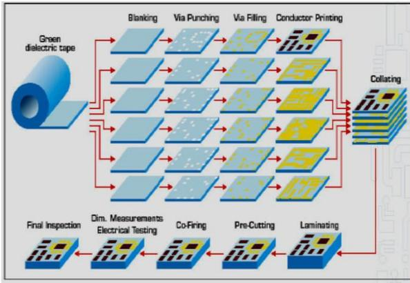
**Figure 1.**Example of LTCC technological line
