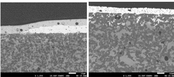
**Figure 3.**LTCC layer (cross-section) with resistive/conductive part above
