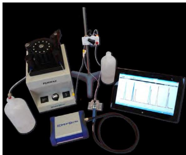
**Figure 9.**Electrochemical test system
