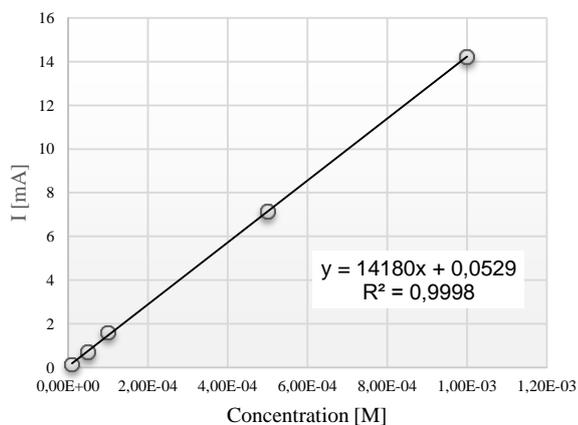
**Figure 11.** Electrochemical test results / calibration curve for Ferricyanide detection
