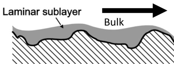
**Figure 1.** Laminar sublayer formation due to roughness
