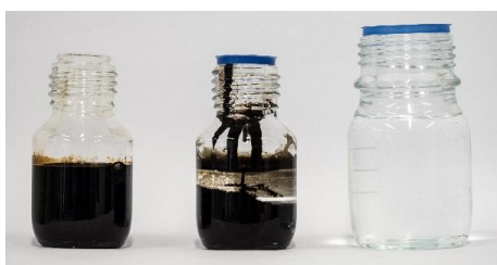
Figure 9: Pure oil (left), bilge water including oil and water phase (middle) and pure tab water (right)
