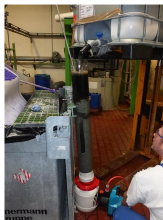
Figure 7. Operational on-road test for the recovery of palladium from industrial process waters by the use of PVAm-modified PET textiles
