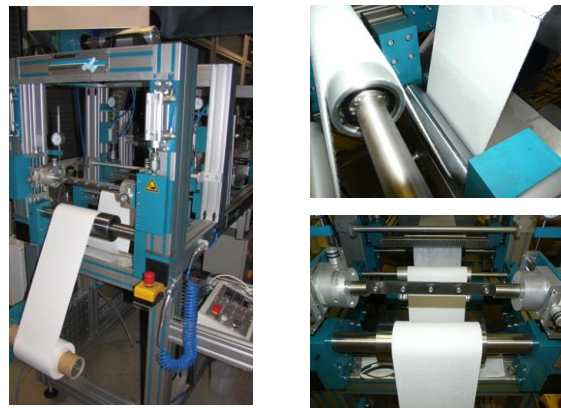
Figure 1. Photographs of the used semi-industrial coating plant for the continuous immobilization of polyvinylamine
