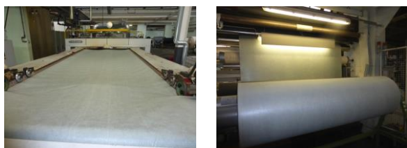
Figure 5. Finishing PET with PVAm on industrial level
